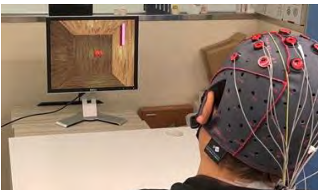
Figure 1: During BCI motor priming. A photo-realistic basketball moved across the screen, from left to right, at a constant rate. The participant was instructed to attempt finger flexion as if they were clutching the ball with both hands. Doing so perturbed the ball's trajectory in the upwards direction. Conversely, resting moved the ball downwards. The goal was to hit the rectangular target.
