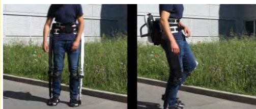
Figure 1. Presentation of degrees of freedoms of autonomy exoskeleton as: Hip abduction/adduction, Hip Flexion/Extension, Knee Flexion/Extension
