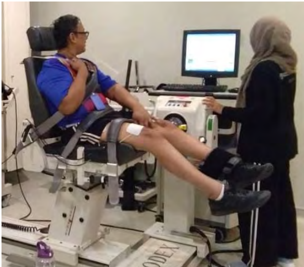
Figure 1: The experimental setup of FES-induced torque data collection by using Biodex Pro 4 Dynamometer and Reha Stim FES. Subject was secured on adjustable chair with his shank in 30 degree knee flexion by dynamometer attachment for isometric test.
